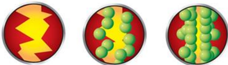
Figure 1. Stages of revitalization in the "metal-metal" friction zone and formation of a protective film [7]
