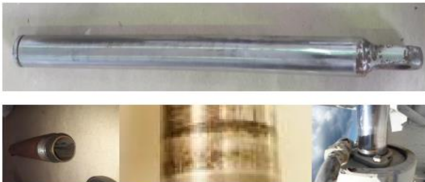
Fig. 1 Appearance of worn surfaces of hydraulic system parts
