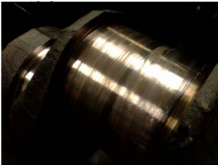
Fig. 1. Seizure of the crankshaft journal.
