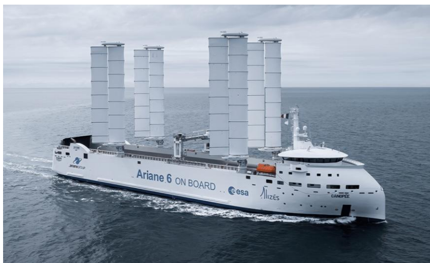
Fig. 1. Wind-assisted container vessel Canopée
