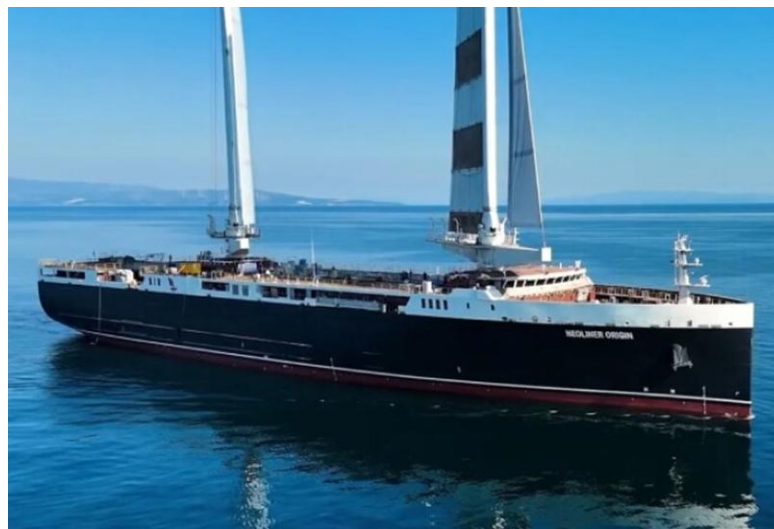
Fig. 2. Vessel equipped with auxiliary wind-assisted propulsion, Neoliner Origin
